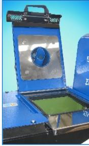
The lid includes a reservoir seal that reduces contamination and insulates molten adhesive.
