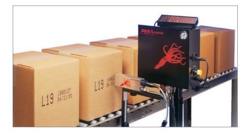
1) The SQ/2 Scorpion utilizes waterbased or solvent-based inks for printing on a wide range of porous and non-porous surfaces. **2)** Run one or two SQ/2 printheads for versatile single line printing.
