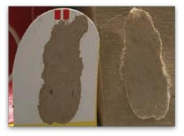
The bonding surface area of the dots provide more adhesion and coverage per square mm of adhesive placed.
