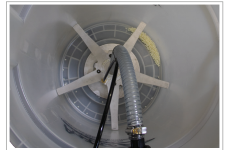
SURE FILL™ FEEDER BIN Bin Shaker to Prevent Adhesive Blocking
